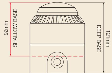
The Flashni is an audible and visual device which requires one single installation point. This greatly reduces installation and costs and is much less obtrusive than two separate devices. Versions are available with the sounder and beacon linked, or with separate terminals for independent operation.
